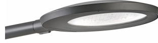
CitySoul gen2 Large - LED module 12000 lm - 830 warm white - Power supply unit with DALI interface - Safety class II - Distribution medium 50 - Clear glass - Gray - Philips standard surge protection level - - Side- entry for diameter 60 mm
