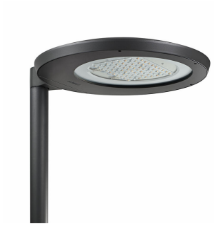
CitySoul gen2 Large - LED module 12000 lm - 830 warm white - Power supply unit with DALI and SystemReady interface - Safety class II - Distribution medium 50 - Clear glass - Gray - Philips standard surge protection level - - - Side-entry for diameter 60 mm
